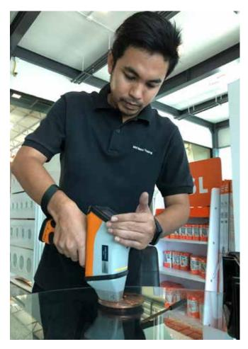
The team also find that the X-MET8000 Expert can clearly address chemical composition of metal, sorting the composition in ascending order, and the metal grade coverage with optional Grade database software is astounding with over 340,000 records. The results from the X-MET have also helped the team to negotiate on selling price where the price is based on the elemental composition of the metal.
