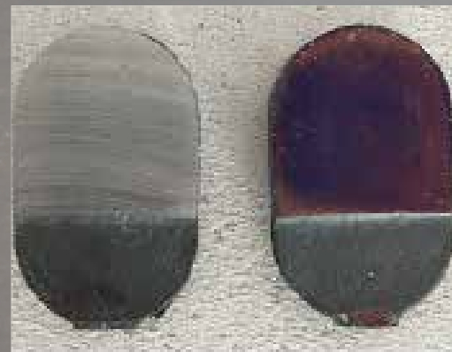
Steel lollipop: ground (left), then heated to 350°C (right).
